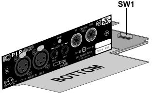
Fig. 3.1 IQ Address Switch (SW1) Location
